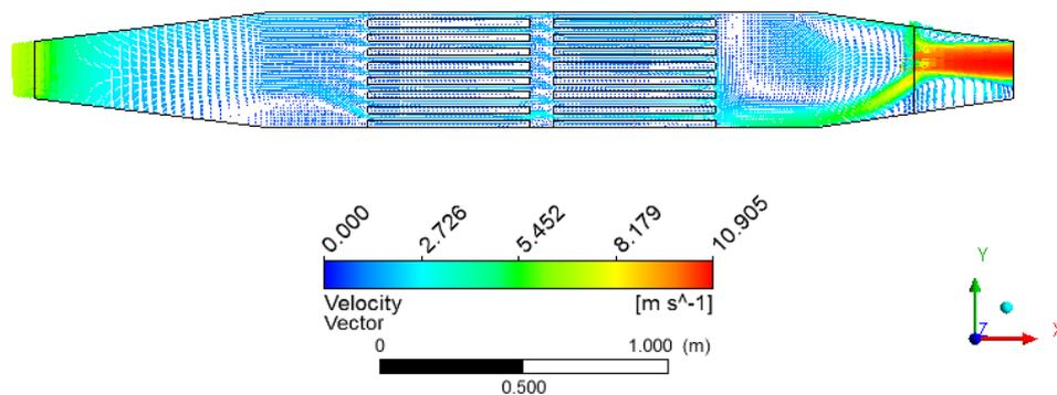
Fig 4: Flow distribution in the modified SCD design with mesh plate in the inlet section
