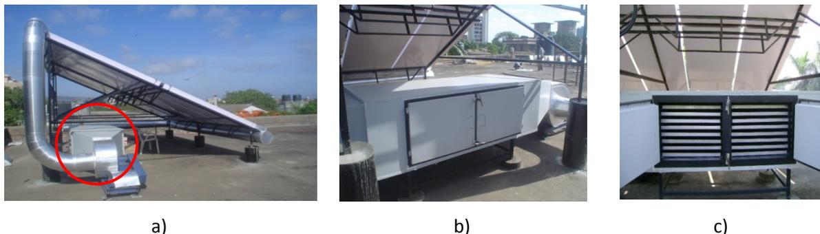
Fig 1: Experimental Set-up – a) SCD with solar panel & centrifugal pump; b) SCD isometric view; c) SCD with two columns of trays
