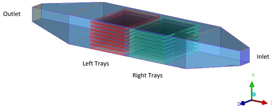
Fig 2: Computational domain of SCD in ICEM-CFD
