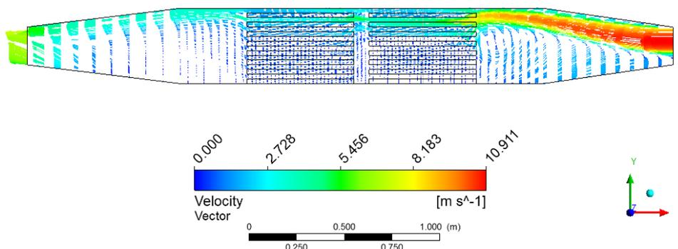
Fig 3: Flow distribution in the original SCD design
